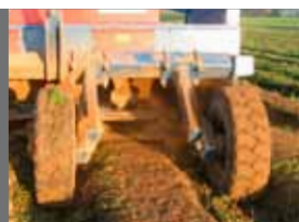
03 Hydraulically driven shakers for the separation of soil
