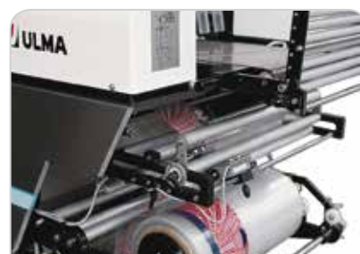
Automatic image centering device for printed film
