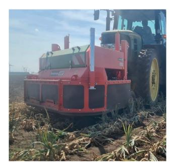
The blade rotors are driven by the tractor PTO via a heavy-duty gearbox and V-belts driven. Depending on 3-point and/or front attachment, the PTO shaft should turn approx. 1000 rpm. rotate.
