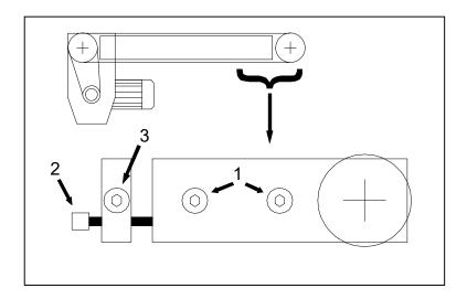
When the belt is not running in the middle of the belt frame and the steering snare in the middle of the belt is coming upwards, adjust 1 side of the adjusting possibility described above.
