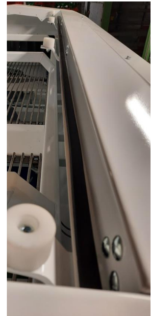
Figure 17. Roof hatch sealing
